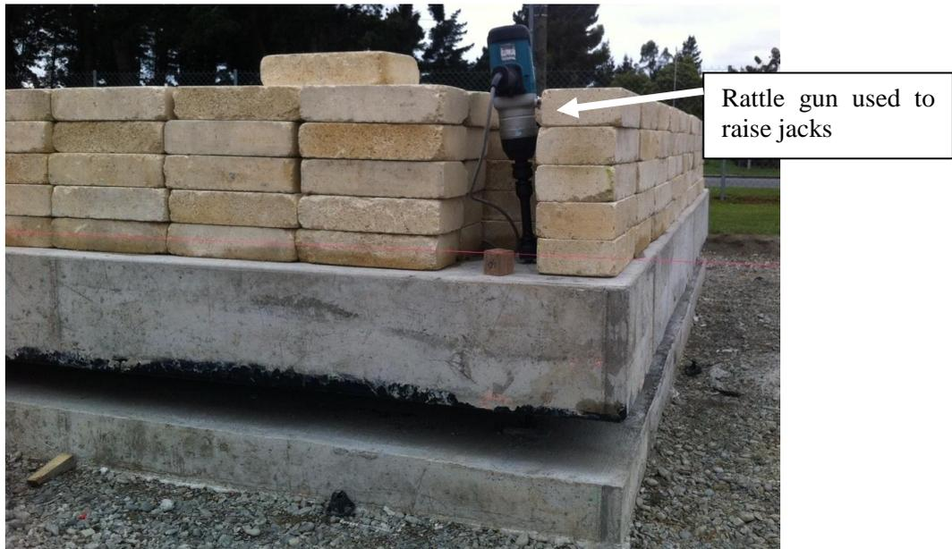
Figure 4 blocks to mimic weight of building cladding, plus rattle gun used to raise slab.
