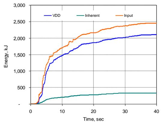
b. Components of seismic energy for elastic structure
