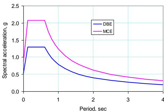
**Figure 5. Seismic demand**
