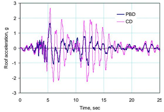
Figure 8. Roof accelerations
