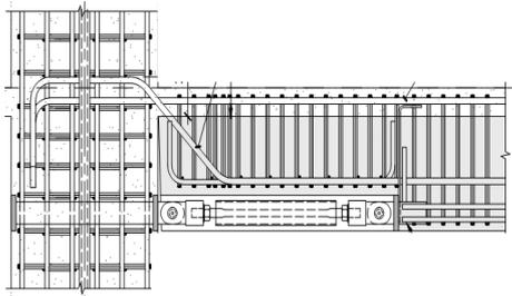
**Figure 8 Elevation of replaceable damper**
