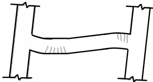
**Figure 4 Cracking pattern in beam due to cyclic action from an earthquake (at “hinge” locations)**
