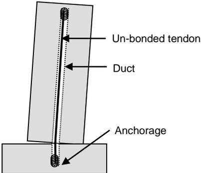
**Figure 2 General components of a rocking wall**
