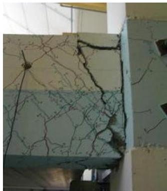
**Figure 6 Monolithic beam column joint (MacPherson, 2005)**
