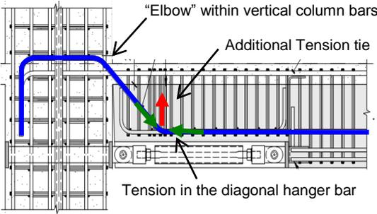
Figure 10 Force components at the “elbow” of the diagonal hanger bar
