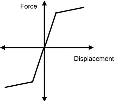
**Figure 3 Non-linear elastic behaviour**
