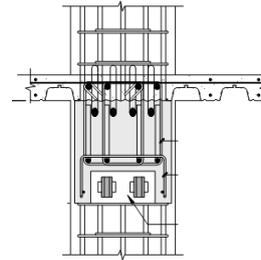
**Figure 9 Section through slotted beam showing replaceable dampers**
