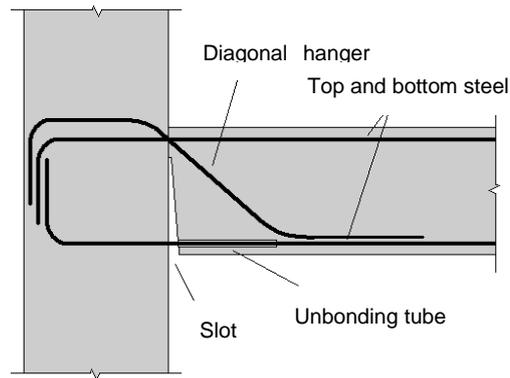
**Figure 5 General arrangement of a slotted beam**
