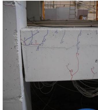
**Figure 7 Slotted beam column joint (Muir et.al, 2012)**
