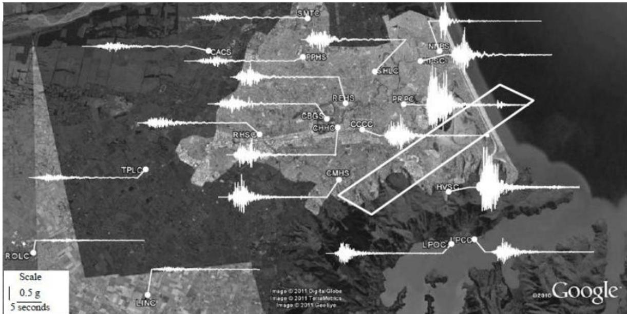
Figure 1. Recorded vertical strong ground motions during the Christchurch earthquake (after Bradley 2012).
