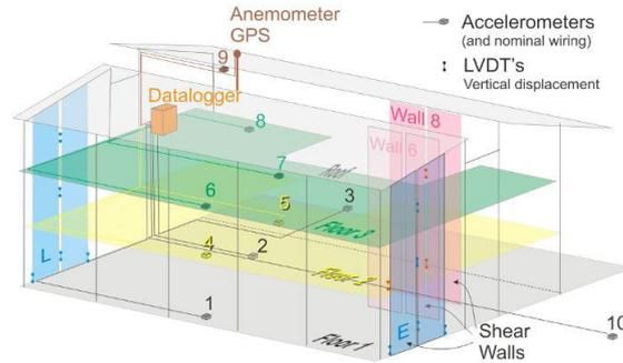
Figure 1 - Layout of sensors in NMIT Arts Building (numbers 1-10 indicate accelerometers).
