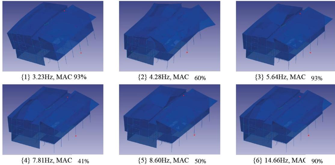
**Figure 2 - Identified mode shapes.**
