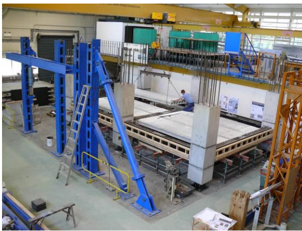
(a) First floor precast components set out.
