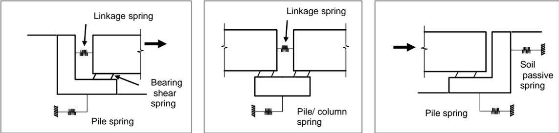
Figure 9. Stiffness elements used in longitudinal response model. Left – pull abutment. Centre – piers. Right – push abutment.
