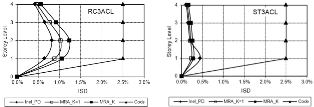
Figure 4 Inter-storey drift profiles for Auckland low-rise buildings
