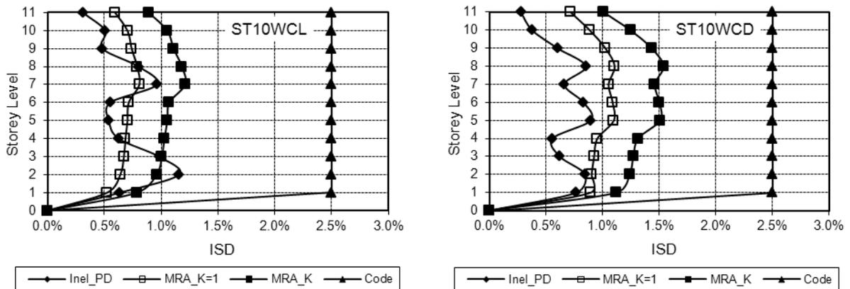
Figure 6 Inter-storey drift profiles for Wellington high-rise steel building
