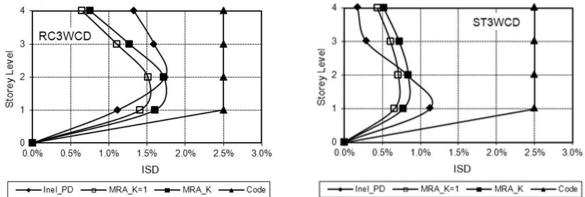
Figure 3 Inter-storey drift profiles for Wellington low-rise buildings
