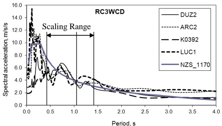
Figure 8 Comparison of response spectra of select records with design spectrum of NZS\_1170
