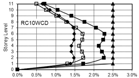
Figure 5. Inter-storey drift profiles for Wellington high-rise RC building
