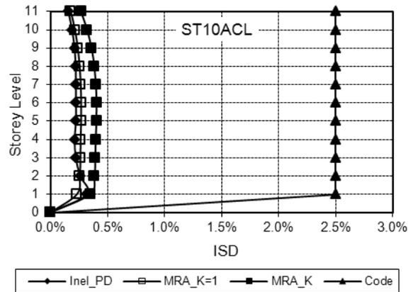
Figure 7 Inter-storey drift profiles for Auckland high-rise steel buildings
