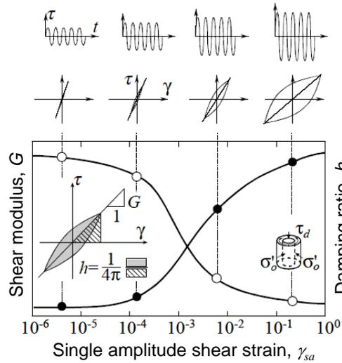
Figure 3. Schematic diagram showing the test procedure and calculation of strain-dependent shear modulus and damping ratio.
