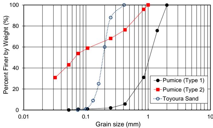
Figure 1. Grain size distribution curves of the samples used in the tests.
