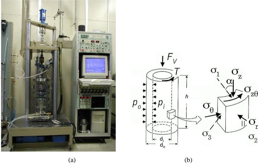
Figure 2. Hollow cylindrical torsional shear tests: (a) apparatus used; and (b) stresses induced in a hollow cylindrical torsional shear element
