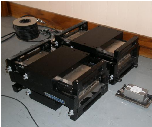
Figure 3 Two long stroke APS Dynamics shakers and an accelerometer
