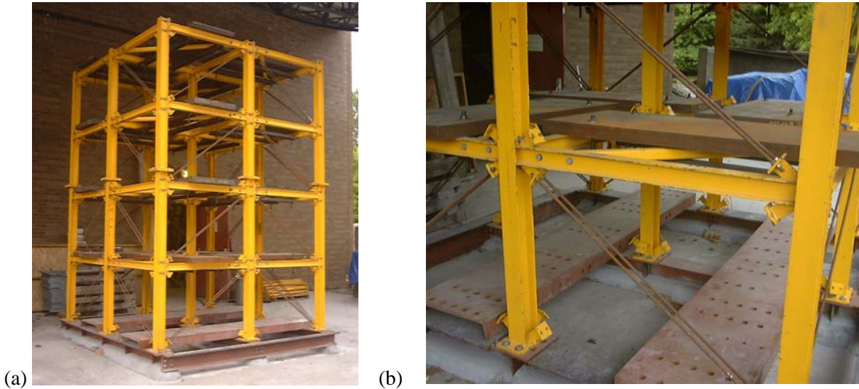
Figure 5. ASCE Phase II Experimental SHM Benchmark Structure: (a) general view, and (b) beam-column joint.
