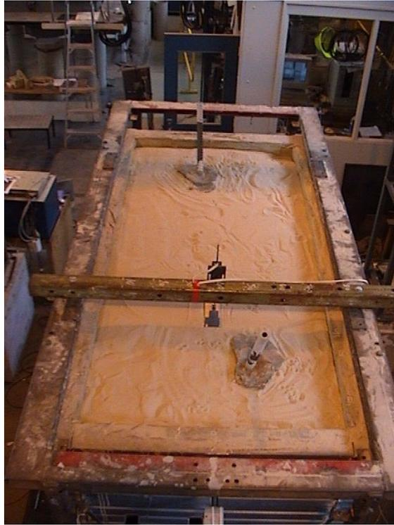
**Figure 8. Completed installation of two inclined micropiles.**
