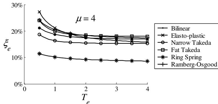
(b) Equivalent damping vs period for displacement ductility  $\mu = 4$
