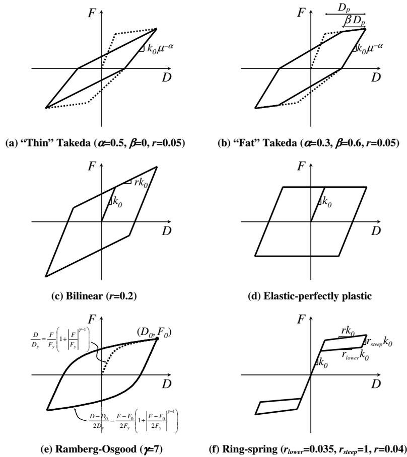
**Figure 7. Hysteresis Rules considered in Direct displacement-based design calibration**
