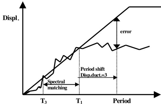
**Figure 4. Displacement spectrum matching for inelastic time-history analysis**
