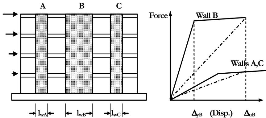
Figure 2. Building with unequal length cantilever walls
