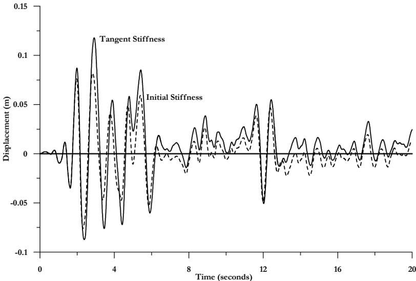
**Figure 5. Displacement response of initial-stiffness and tangent-stiffness SDOF to El Centro 1940NS**
