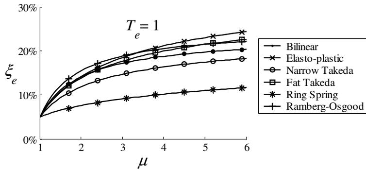
(a) Equivalent damping vs ductility for effective period  $T_e = 1.0$  seconds
