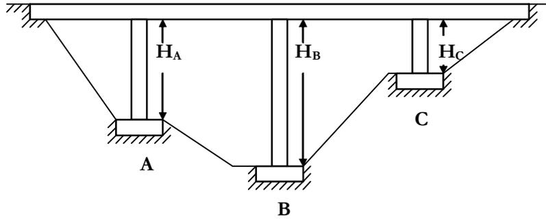
**Figure 3. Bridge with unequal column heights**
