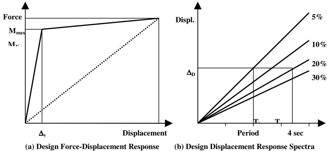
**Figure 1. Essential differences between force-based and direct displacement-based design**
