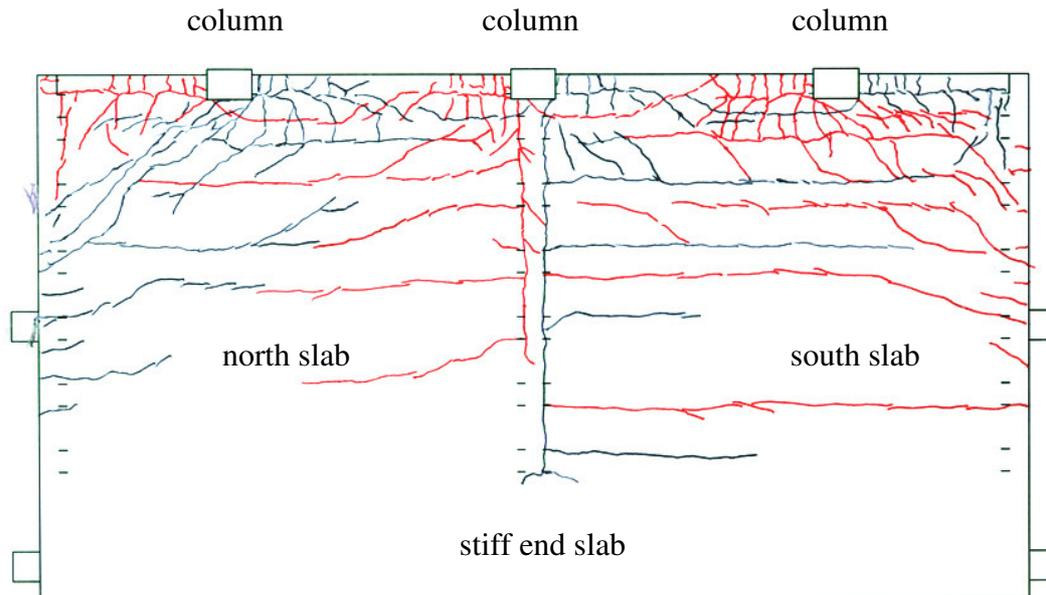
Fig. 7: Crack pattern in floor slab at 3% drift.
