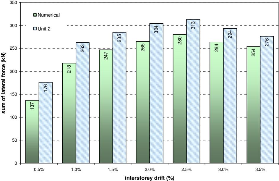
Fig. 10: Comparison of Experimental and Numerical Force versus Deflection Response
