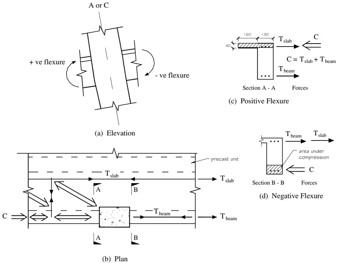
Fig. 5: Strength increase for beam at columns A & C.
