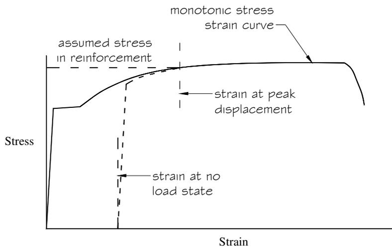
Fig. 8: Assessing stress levels in reinforcement crossing cracks (d – e and f – g)
