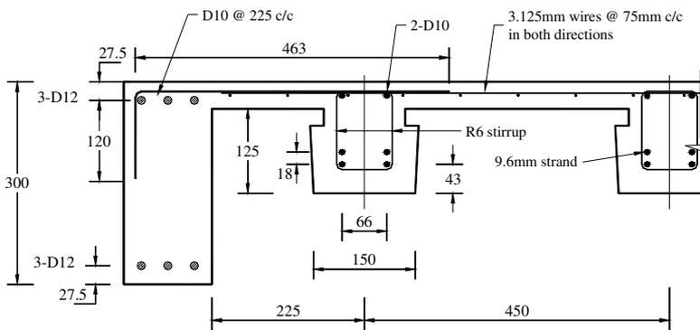
Section A - A: Main Beam and Floor Slab
