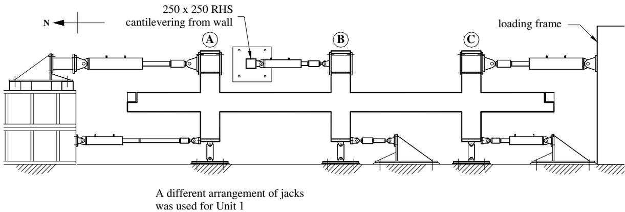
Fig. 2: Schematic of test arrangement for Units 2 and 3.
