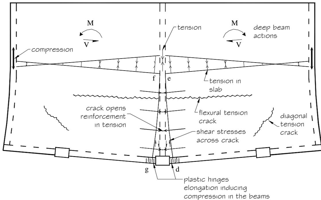
Fig. 6: Floor slab acting as a deep beam due to elongation in plastic hinge regions.
