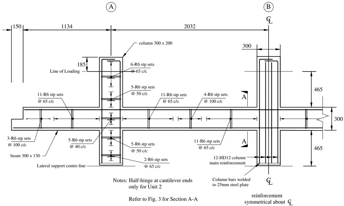
Fig. 1: Details of reinforcement in all three frames.
