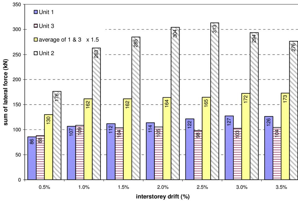
Fig. 4: Lateral shear resisted by frames at peak displacements in positive direction.
