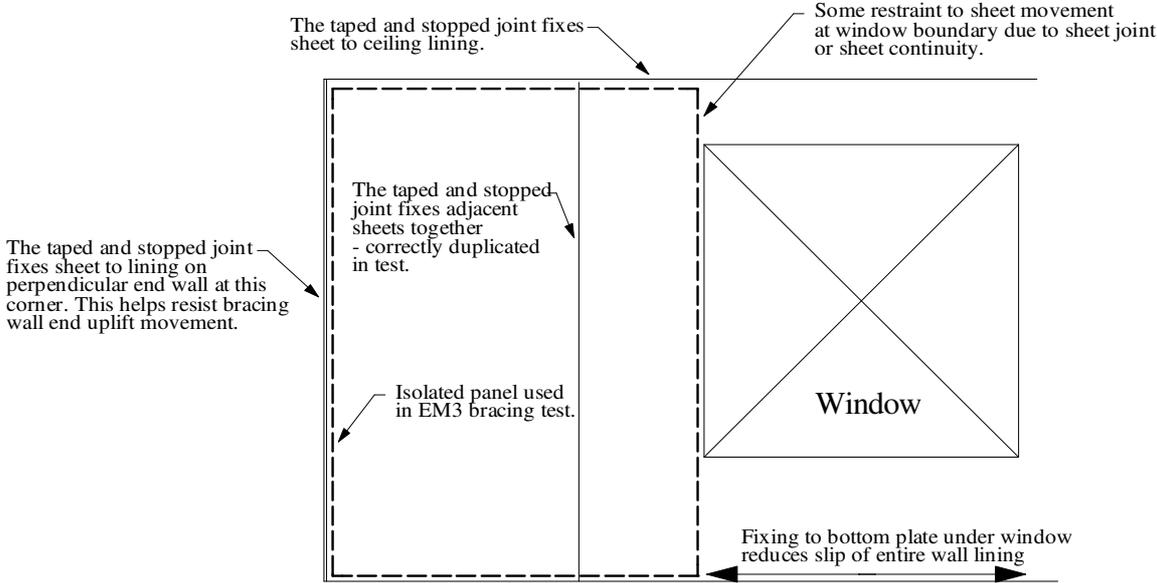
**Figure 3. Restraint of wall lining in real buildings**
