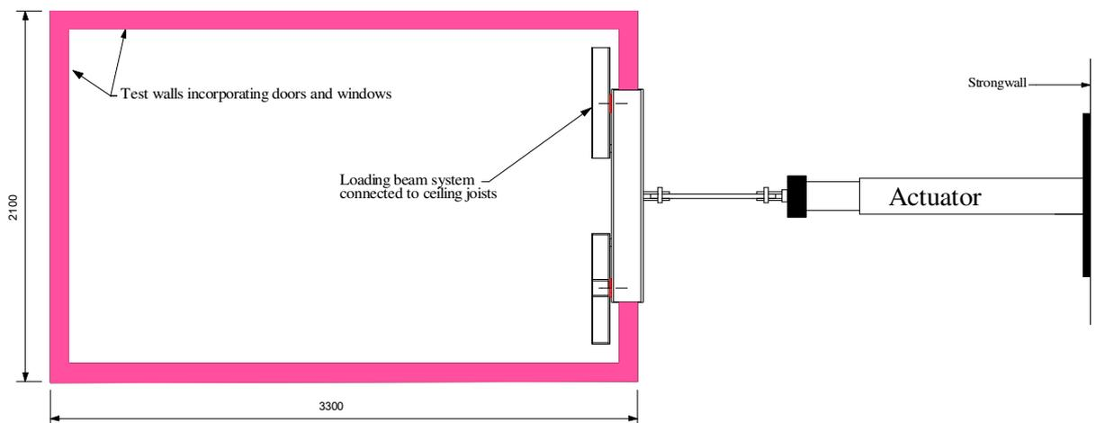
**Figure 5. Room racking test – foundation beams and loading system**
