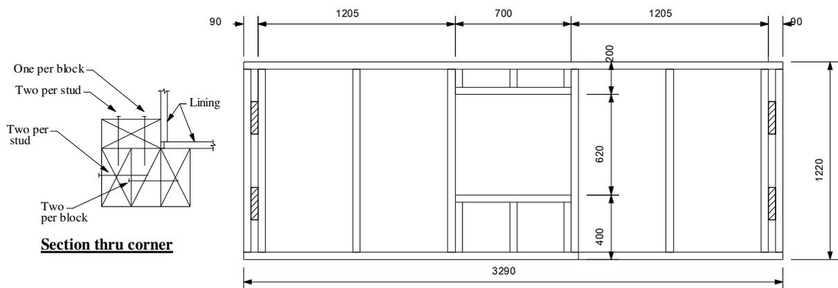
**Figure 6. Room racking test – timber framing side walls**
