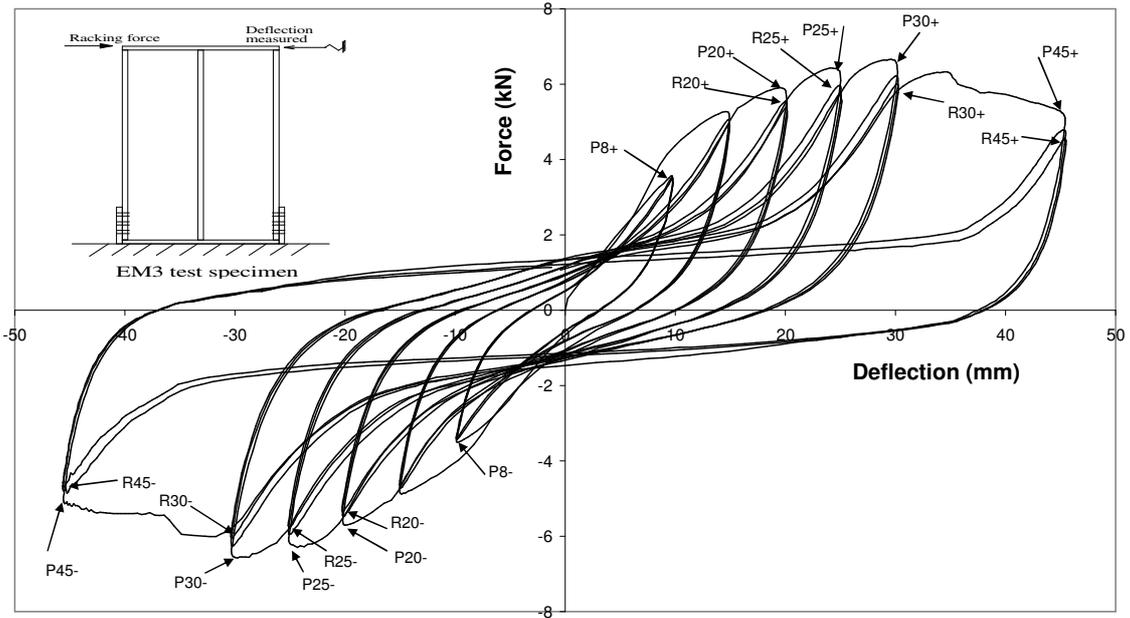
Figure 2. Hysteresis loops from an EM3 test
