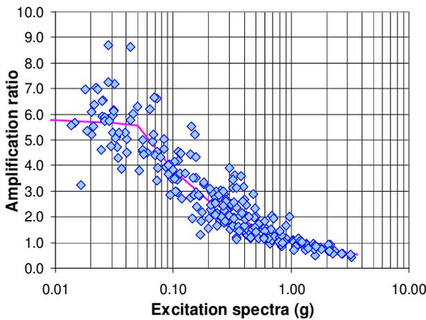
Figure 15 Amplification ratios for 0.2s period. The soil line is the fitted function of excitation spectra
