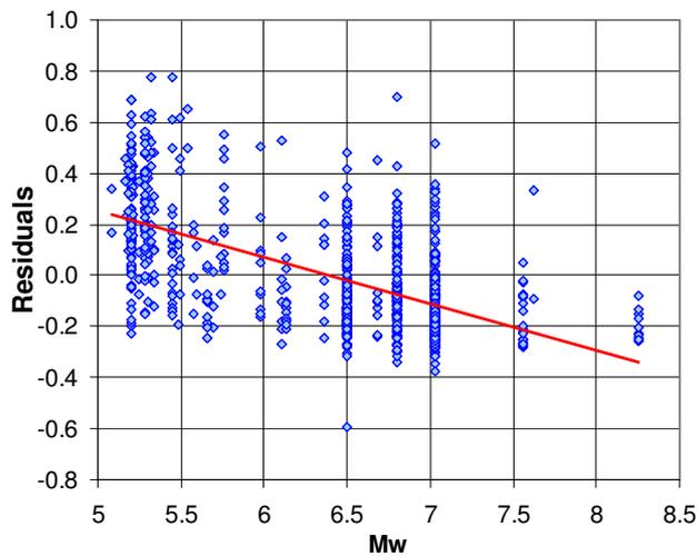
Figure 5 Residual distribution with respect to magnitude at 3s period for a 0.75s elastic 1-D soil
