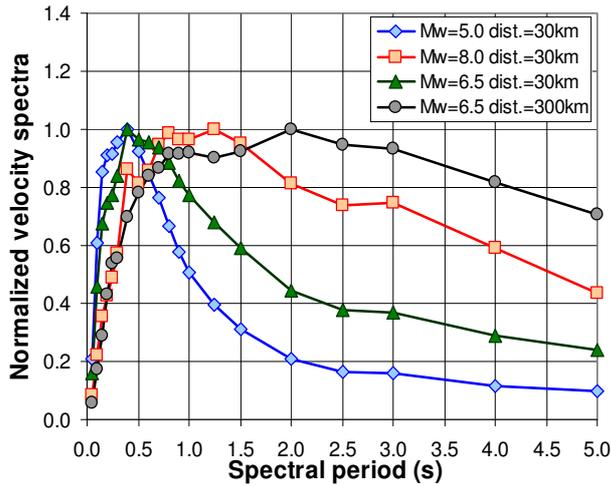
Figure 1 Spectral shape for different magnitude and source distance from an attenuation model
