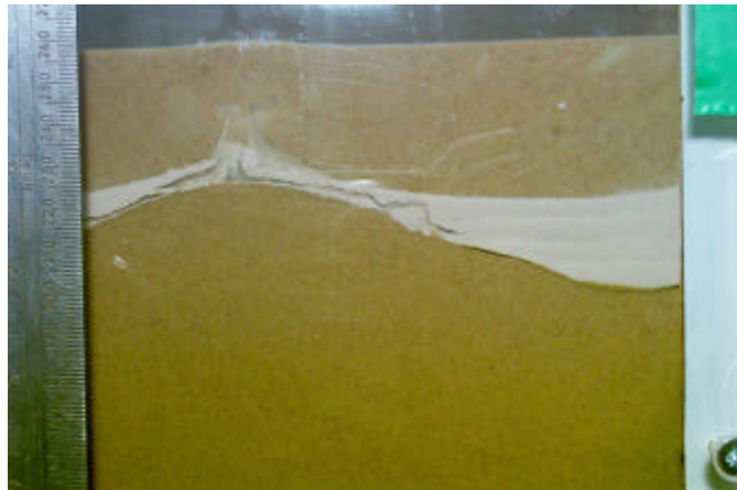
Figure 3c, Test D. The silt layer fails and two plumes of water surge toward the surface.
