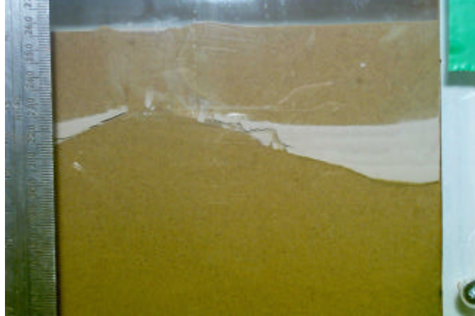
Figure 3e, Test D. Between 1 and 2 minutes later the water pressure has dissipated completely. Post-liquefaction settlement of 1.0mm for Test D. Total combined post-liquefaction settlement for Tests A (0.4g), B (0.4g), C (0.3g) and D (0.6g) is 5.7mm.
