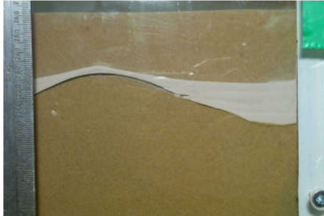
Figure 2b, Test.A. The soil has completely liquefied and settled. Maximum water film thickness of 1.1mm.
