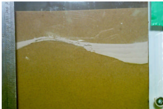
Figure 3a, Test D. Hydraulic equilibrium before the \sim 0.6g shake. The sample has been tested 3 times before and the silt layer is visibly damaged.
