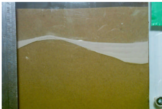
Figure 2c, Test A. The water pressure has dissipated through or around the silt layer, a process which took between 10 and 30 minutes. Total post-liquefaction settlement of 2.0mm.
