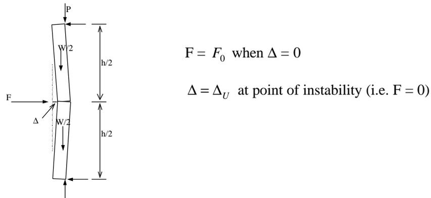
Figure 2. Diagram for static rigid-body analysis of URM wall.
