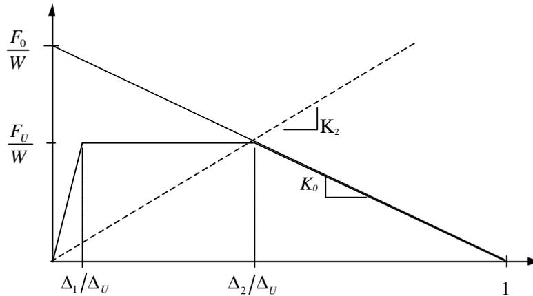
Figure 1. Generic tri-linear force-deformation relationship for URM walls.
