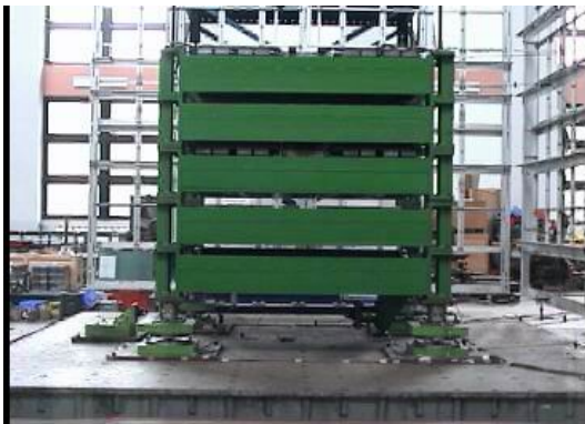
Figure 5 Shaking table test for 5-layer structure
