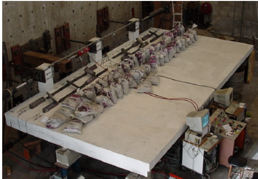
Figure 1: Frame with floor slab test unit.
