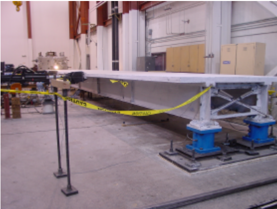
Figure 1. Bridge model with actuators applying pseudo-static transverse loads
