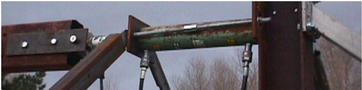
(d) Hydraulic jack, load cell and connection to reaction frame.
