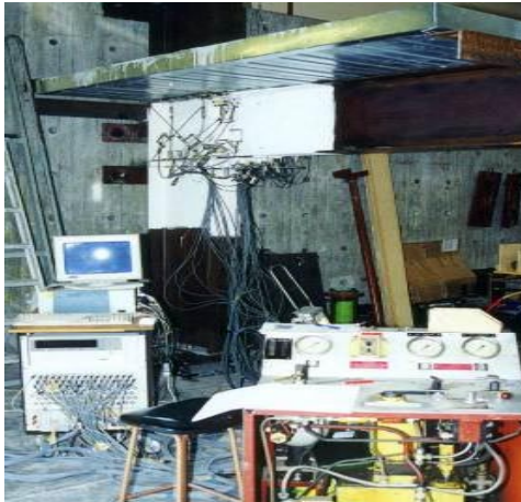
Figure 7 Large-scale SHJ test 3 showing set-up of specimen and floor slab
